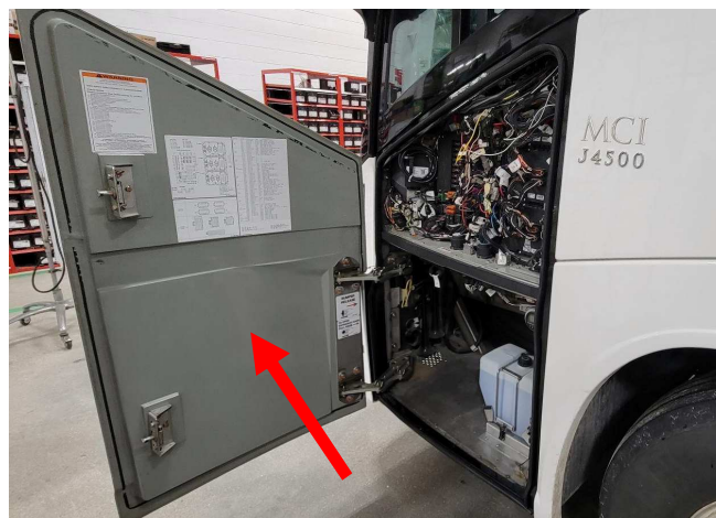
Figure 2: Left side forward access door
