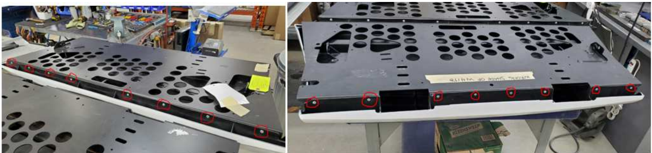
Figure 10: Remove rivets from the inner frame of the bumper
