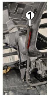
7. Install wiring harness into 70 mm length of corrugated tubing. The location is approx. 30 mm from the support clip show in the example photo. Install the piping in the area indicated by the red line. Using abrasion resistant tape to secure both ends of the tubing to the harness and install wiring back into proper position.
