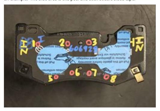
To apply the paste correctly, the pads must be removed from the calipers. See the photo below for an example of what the front brake pads look like once they have been separated from the caliper pistons.
