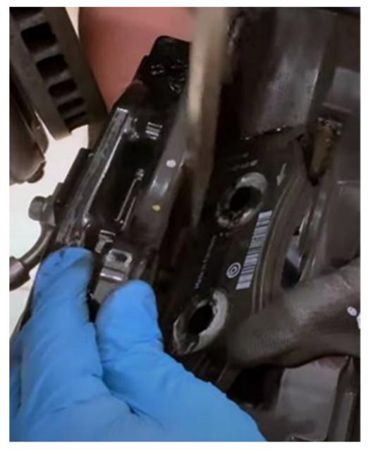
This is normal when the front pads have been removed. When this has been done, remove as much of the remaining tape residue as possible. Then, apply the copper paste as directed in the bulletin. Once the copper paste has been applied correctly to the front brake pads, simply reinstall them into the calipers. There is no need to replace the front brake pads during this service because of the double-sided tape.
