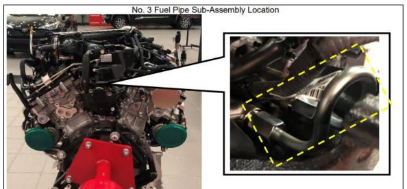
If this condition is identified, it is important to check for debris in the LH No.2 Fuel Delivery Pipe and No.3 Fuel Pipe Sub Assy connection port to help eliminate any repeat repairs for customers. Please create a TAS case and contact TAS for instruction prior to diagnosing or repairing of the vehicle. Please save all parts and/or details and submit a field report.
