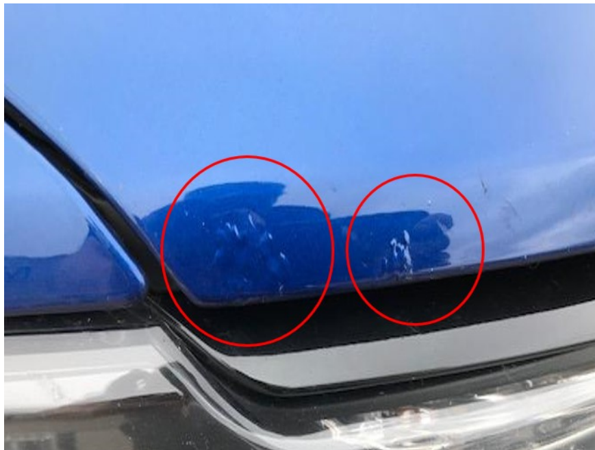
Fig. 3 Examples of Corrosion Along Leading Edges
