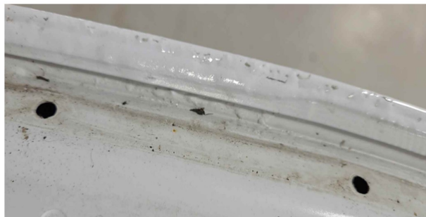
Fig. 1 Hem Flange Area Example
