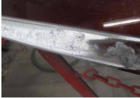
Perforation/Pitting Found After Sanding Examples (Fig. 1)
