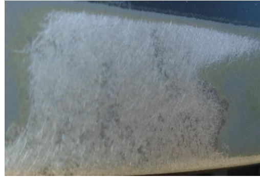
Perforation/Pitting Found After Sanding Examples (Fig. 1)
