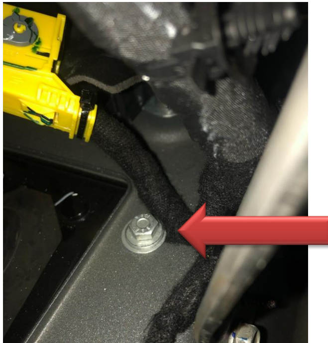
Wiring Harness Crushed Under Bolt
