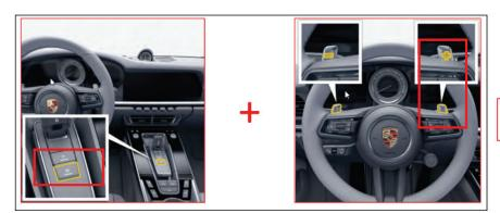
Upshift from 1<sup>st</sup> 2<sup>nd</sup> Gear is restricted in Manual Mode.
