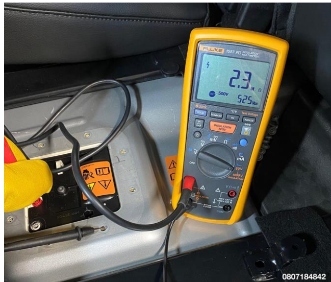
Figure 28 – Measure and Record Isolation Resistance Between HV Positive Test Point and Chassis Ground
