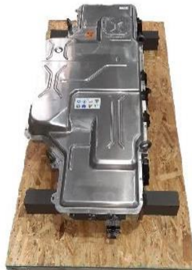
Figure 26 – HV Battery on Top Cover
