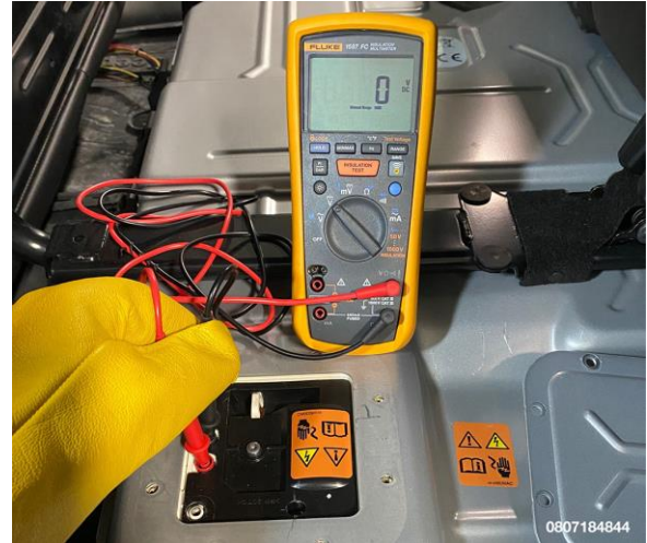
Figure 5 – Measuring at High Voltage Test Points
