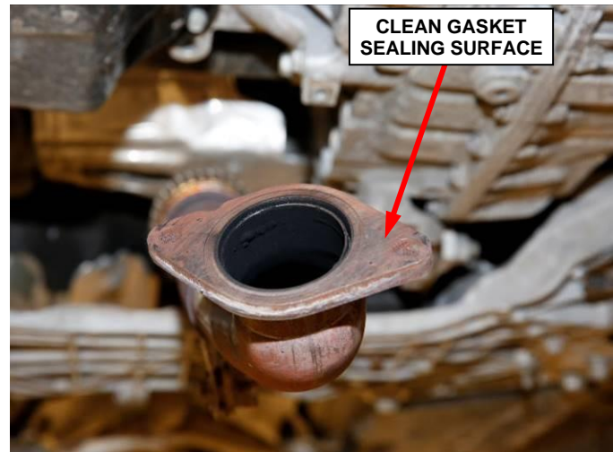
Figure 25 – Crossunder Pipe Flange
