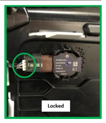
If the sensors are correctly installed and connector locks are engaged check for DTCs and continue diagnostics. Inspect pins on sensors. Connector repair kits are available if bent pins or connector damage is found.
