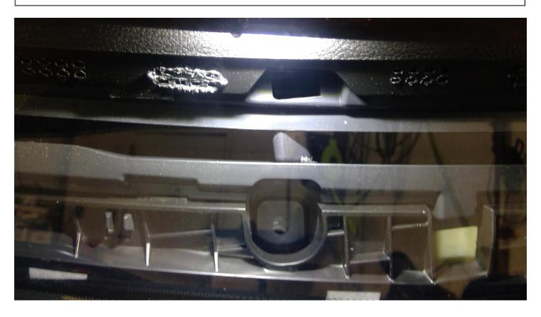
Fastener part number 06100567 attaches the upper dash to the body at the windshield.
