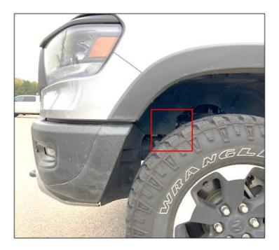
**Discussion**: If a customer states there is a rubbing, clunking, or rattle noise on tight turns while cornering, inspect the above area for signs of contact with the tire. If rub marks exist on the splash shield it is not necessary to replace it. Using hand pressure over bend and adjust the shield away from the tire in the diagonal area shown in the image below.
