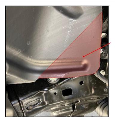
Once the adjustment is completed test the fitment by turning to each steering lock to confirm the improvement in clearance.
