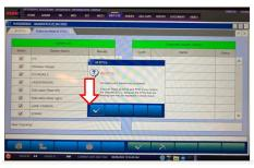
**IMPORTANT:** The "Erase and Read all DTCs" must be performed since DTCs may be generated and stored.
