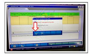
**Note:** Do not disturb the cable or turn off the ignition during reprogramming to prevent damage to the ECU.
