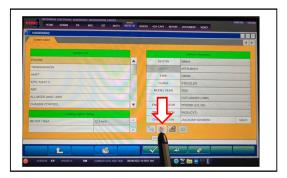
**IMPORTANT:** The "Erase and Read all DTCs" must be performed since DTCs may be generated and stored.
