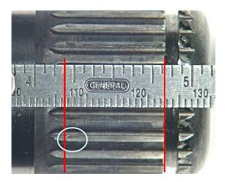
1. Remove the left side front wheel drive shaft, take a clear close up picture of the spline indicating engagement at 16 mm at the end of the groove to the end of the spline, as shown in the picture above. Refer to Front Wheel Drive Half Shaft Replacement - Left Side in SI.
