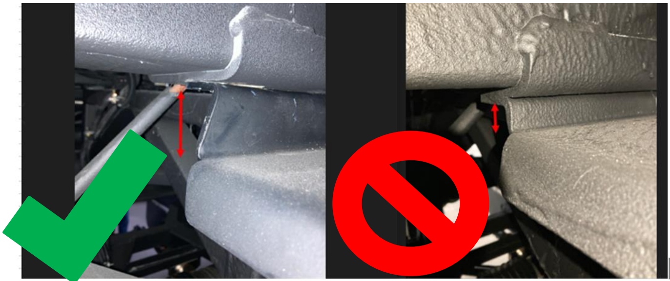
Figure 1: Correct Flange Height of Tag Axle Air Spring Mounting Brackets for J Model Coaches = 2.26"
