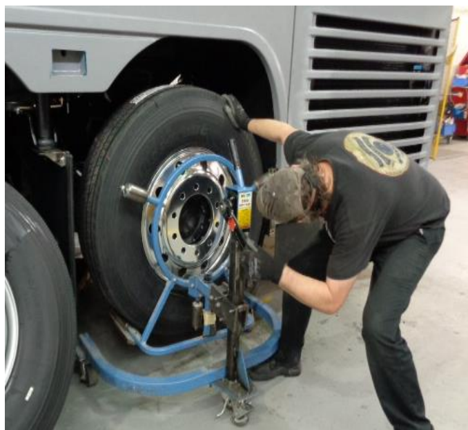
Figure 3: Remove Tag Axle Wheel
