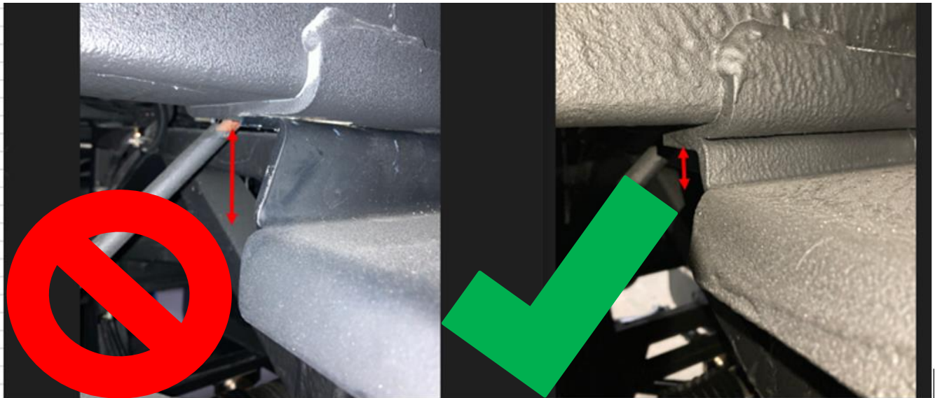
Figure 1: Correct Flange Height of Tag Axle Air Spring Mounting Brackets for CRT Model Coaches = 1.21"
