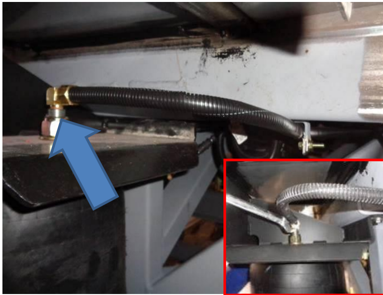
Figure 4: Disconnect Air Line
