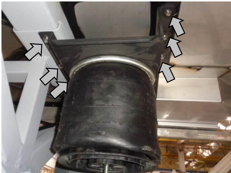
Figure 5: Unfasten the Tag Axle Air Spring Assembly
