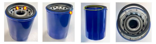
If any damage is found, replace the filter. If no damage is found, the seal may be refitted to the filter and installed on the vehicle.
