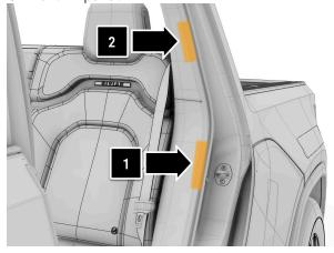
Tip: Pull back the secondary door seal as necessary to insert the inflatable wedges.
