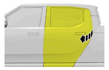
2. Use the inflatable wedges in the highlighted areas to gain access to the forward clips on the LH upper C-Pillar trim panel.
