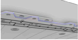
**Tip:** Attach a flexible straw and use an inspection mirror to apply sealant to tight areas. Working in small sections will allow the sealant to be spread without curing.
