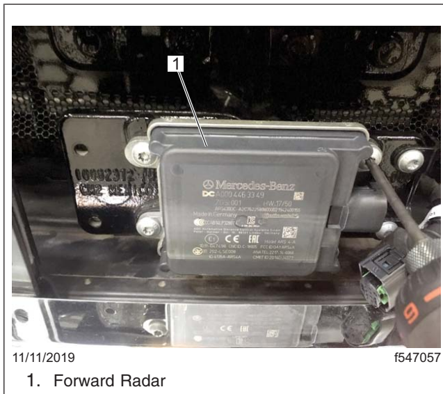
Fig. 3, Forward Radar Removal
