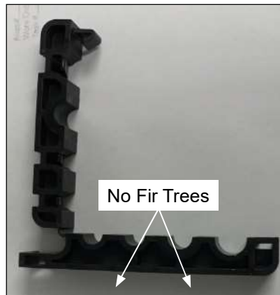
Figure 1 — Incorrect Bracket, Without "Fir Trees"
