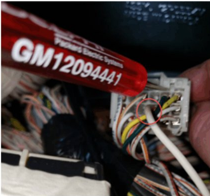
22. Release the locking tab on the new jumper harness.
