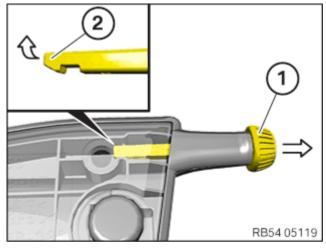
• Lever out the quick-release axle (1) for the wind deflector with a suitable tool at the retaining lug (2) and feed out in the direction of arrow.
