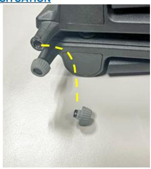
It is possible that the guide stem (aka rotational axis) on the wind deflector can break, upon removal and or during installation.
