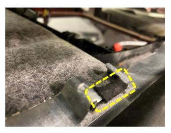
3. Cut felt strips to 20 mm x 10 mm dimensions and apply it to all the brackets on the headliner (shown).
