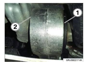
The bushing in the lower engine stabilizer link (1) is working its way out of its aluminum housing.
