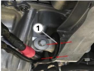
There can be up to a 2 mm gap in the bushing and the stabilizer link (1). Only replace the link if it is in actual contact with the oil pan.
