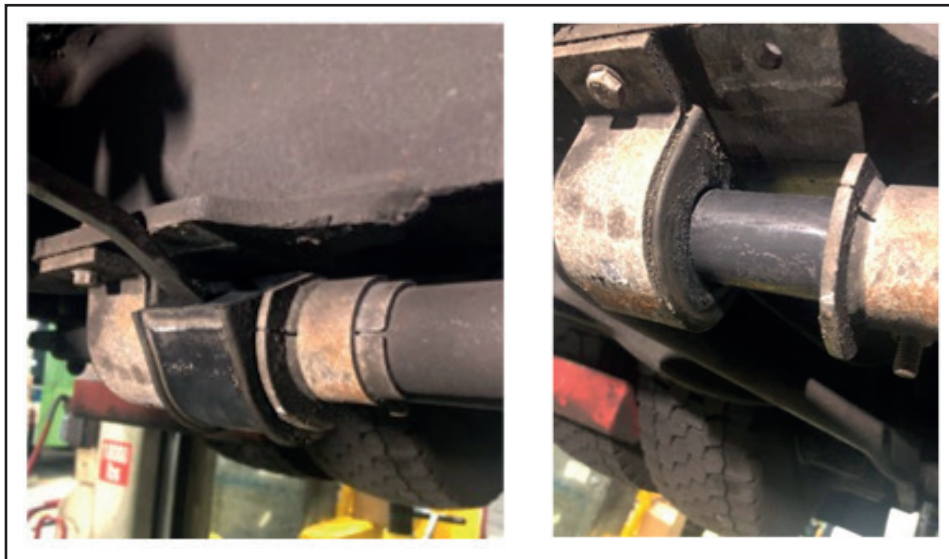
Figure 27 - Typical View of Damaged Bushing
