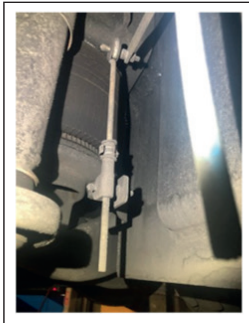
Figure 17 - Location of Rear Leveling Valve
