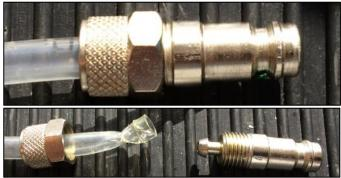
2. Attach the compression fitting to the tubing on the new nozzle assembly.
