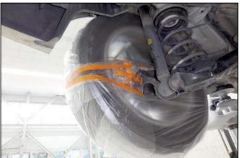
Wrap the exhaust areas adjacent to the front sub-frame and the rear Coupled Torsion Beam Axle (CTBA) with plastic bags to protect them from overspray. Use tape to secure the plastic in place.
