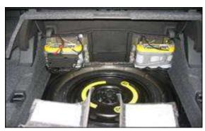
(3.2L) Test/charge AGM battery located in trunk - one 6V battery located on each side of ski chute, as shown.
