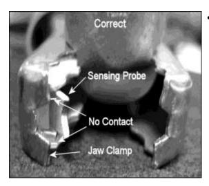
There must be no contact between the inside connection and outside jaw of clamp -arrows-.
