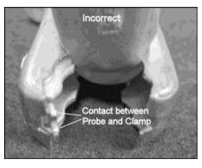
• Inside connection is bent and touching outside of the clamp, -arrows-.
