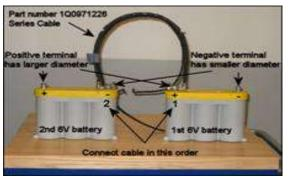
Connect cable (Part No: 1Q0971226) to inner battery terminals.
