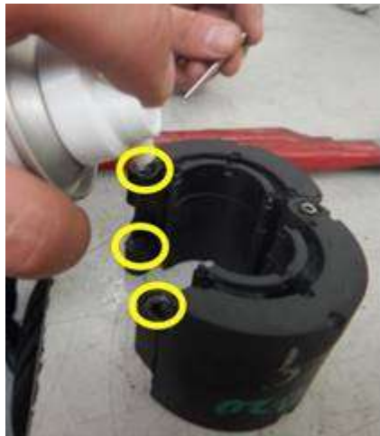
Figure 1. Lubricate pin holes of the damper weight in marked locations.
