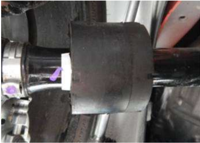
Figure 6. Final positioning of damper weight without screw clamp.
