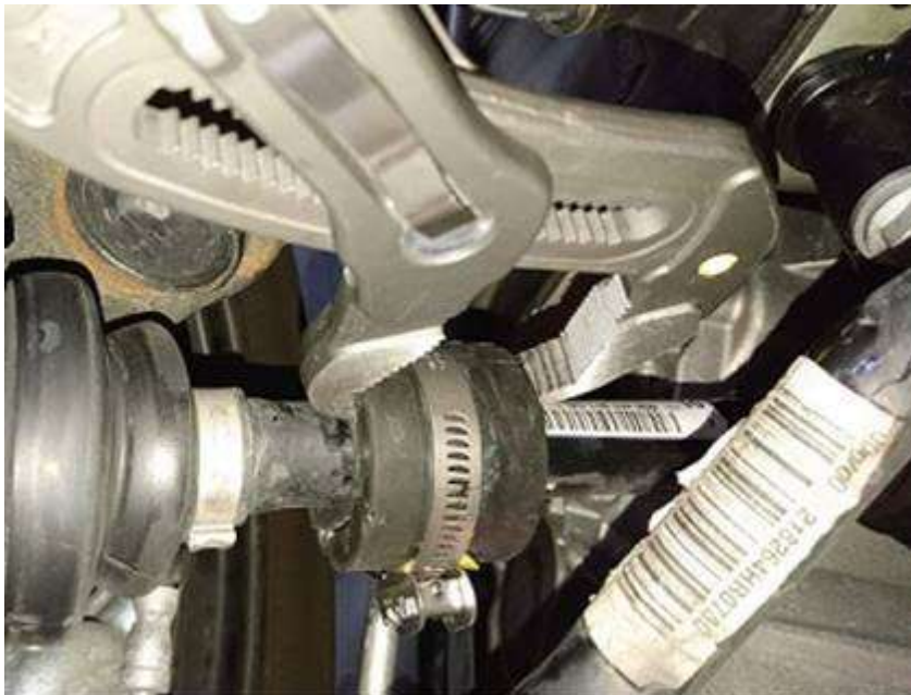
Figure 5. Pressing of the hold-down pin into the damper weight.
