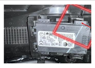
Example of a Mid Range Rear Radar not fully snapped in
