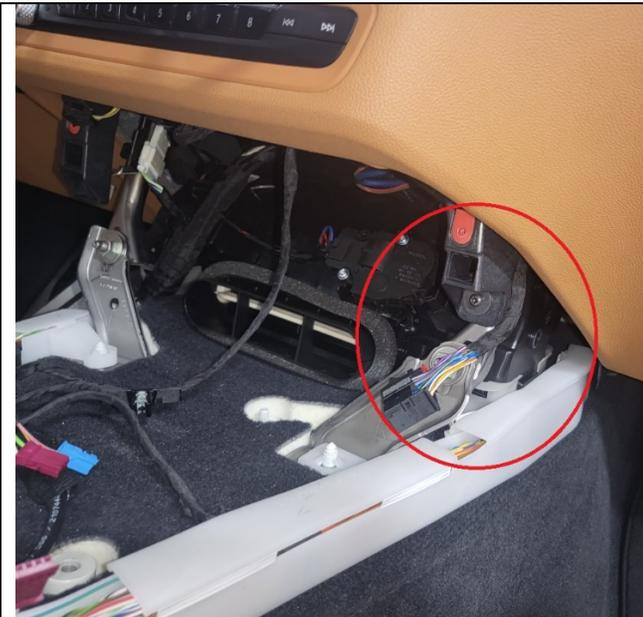
5- Apply felt tape to the location pictured on the passenger side.
