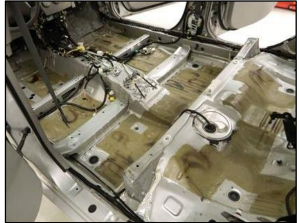
Figure 13. Example of Vehicle With LASD Removed Using Plastic Scraper and Heat Gun
