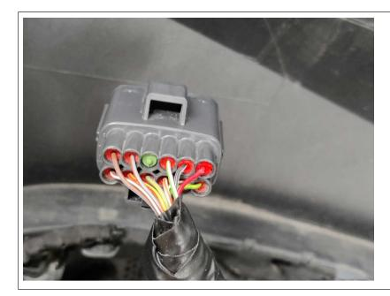
Locate and disconnect the FMDM wires using the wiring diagram.
