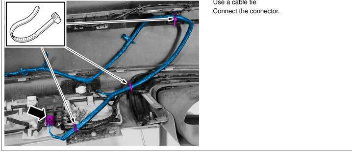
Reinstall the removed parts in reverse order.
