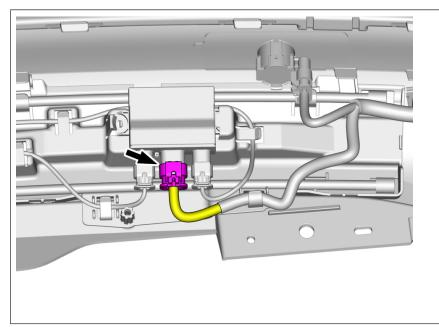
Disconnect the connector. Fold the cable aside.
