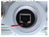
This will reset the device to factory defaults and reboot. Please be patient as this could take up to 5 - 10 minutes. If the reset resolved the issue, then the light of the LED will finally switch to either green or blue.
