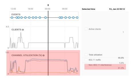
**Recommendation to workshop:** The following devices can also cause RF interference degrading the performance of the wireless network. These devices should be kept as far as possible from the workshop area:
