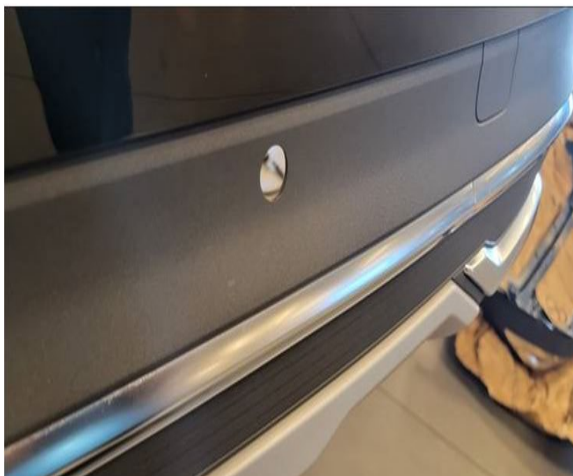
Figure 1: The parking aid mount has come loose.
