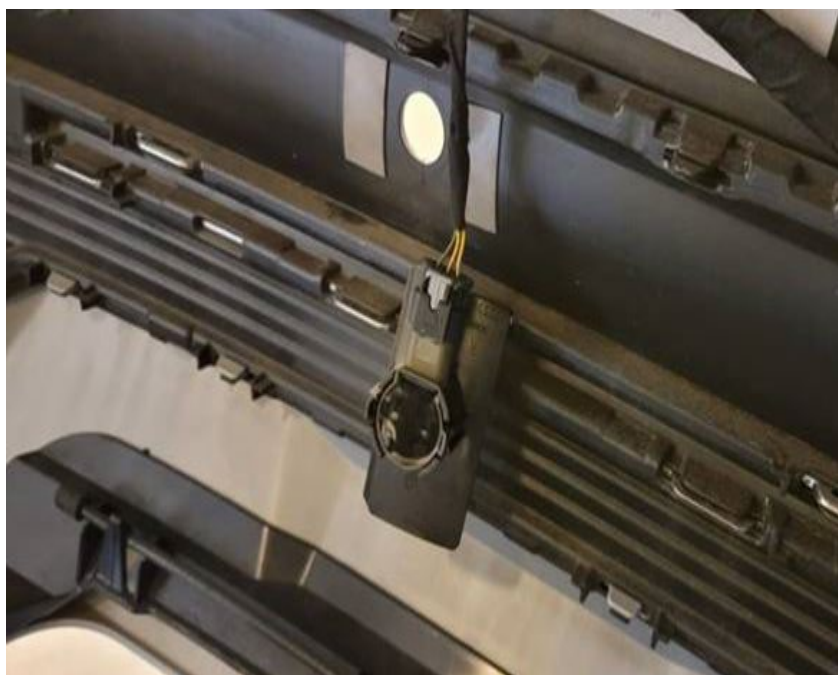
Figure 2: The parking aid mount has come loose.
