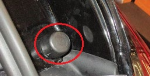
Figure 1. Check the adjustment of the bumpers/buffers and apply special lubricant.
