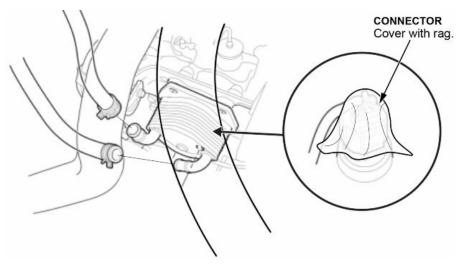
83. Install the shift cable on the transmission side.
