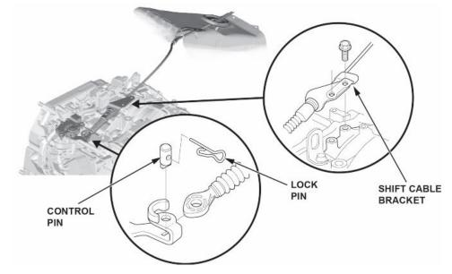
NOTE: Make sure the control pin is inserted through the shift cable end and fully seated on the control lever.
