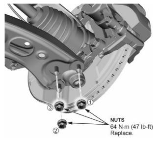
66. Connect both sides with the stabilizer link ball joint.
