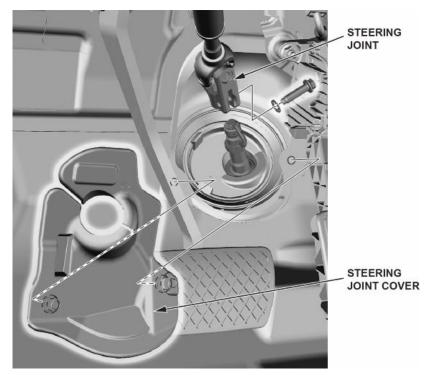
• Hold the lower slide shaft on the column with a piece of wire between the joint yoke of the lower slide shaft and joint yoke of the upper slide shaft to prevent the lower slide shaft from pulling out.
