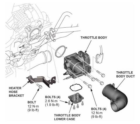
85. Install the throttle body inlet pipe.
