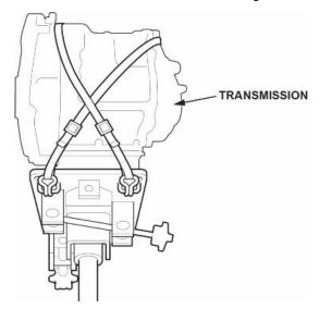
56. Install the lower transmission assembly mounting bolts.
