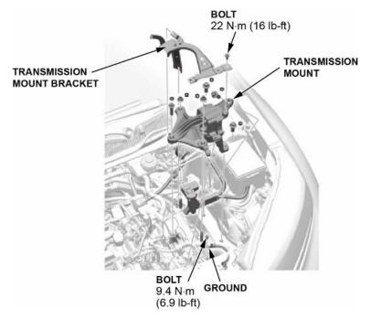
72. Install the upper transmission assembly mounting bolts.
