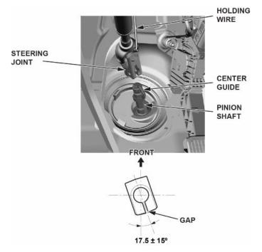
93. Install the steering joint bolt and cover.
