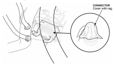
17. Remove the intake air resonator.
