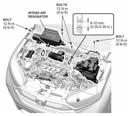
18. Remove the engine wire harness bracket.
