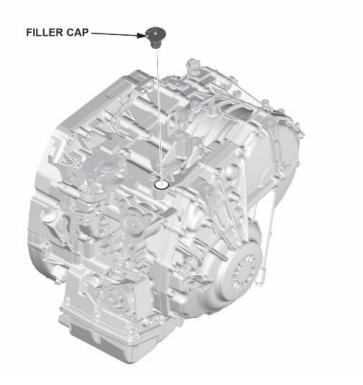
96. Check the transmission fluid level.
