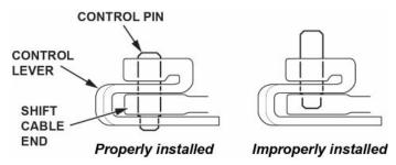
NOTE: Make sure the lock pin is inserted through the control pin hole to the opening of the control lever so that the hooked end of the lock pin locks into the control pin hole.
