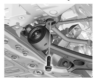
65. Connect both sides of the lower arm ball joint.
