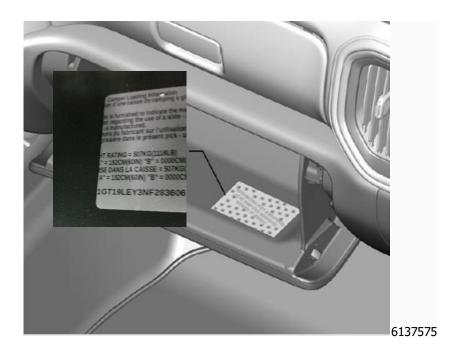
Remove the misprinted camper label (shown above in glove box) and any residue using isopropyl alcohol and dry
