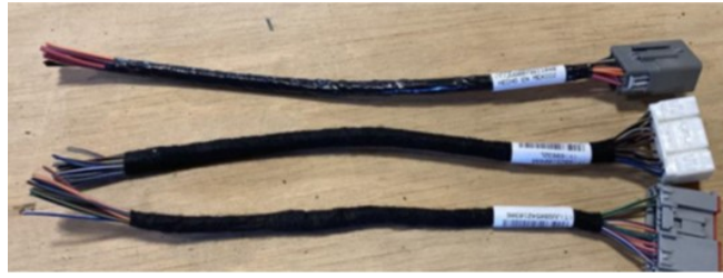
Fig. 1 Three VSIM Wiring Jumper Harnesses
