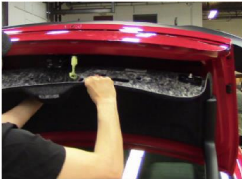
Figure 4 – Decklid Liner Removal
