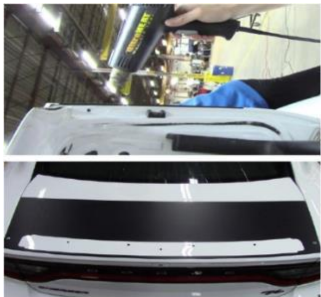
Figure 17 – Applying Heat to Edges
