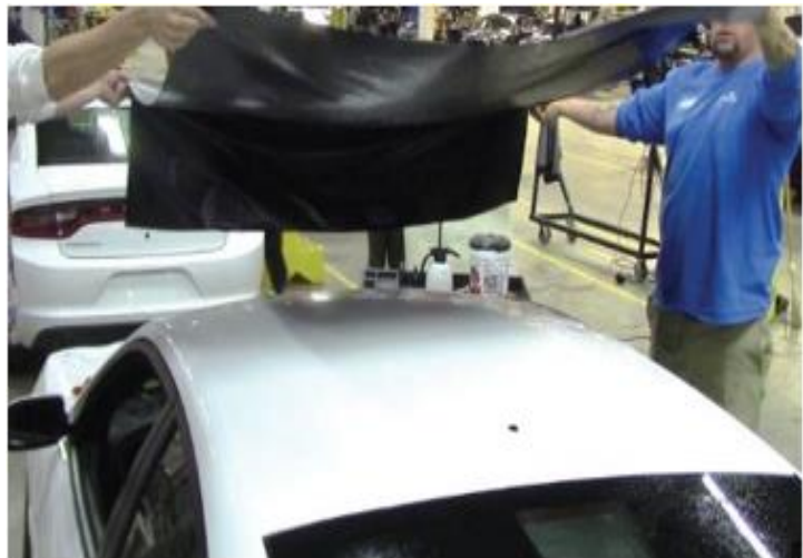
Figure 48 – Roof Decal Installation
