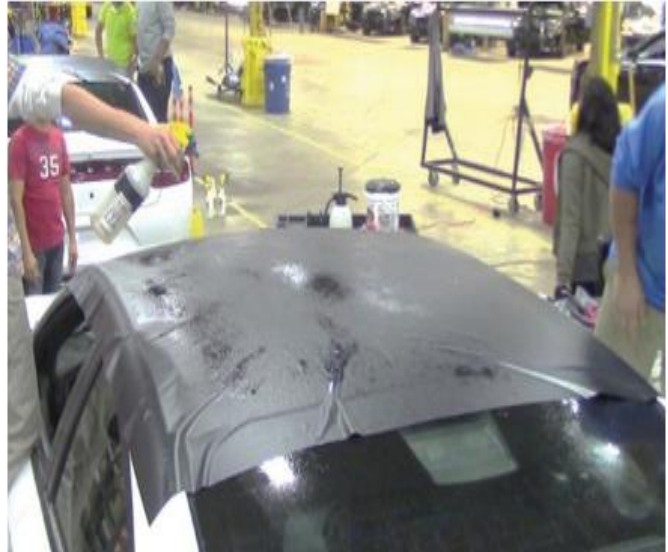
Figure 50 – Spray Roof Decal
