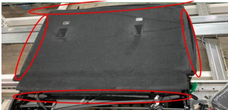
Loose fitment of cover in areas shown.
