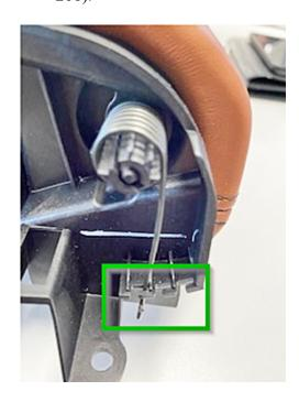
2. Inspect and adjust the spring's end (shown) on the "slow" door to match the speed of normal operating door.
