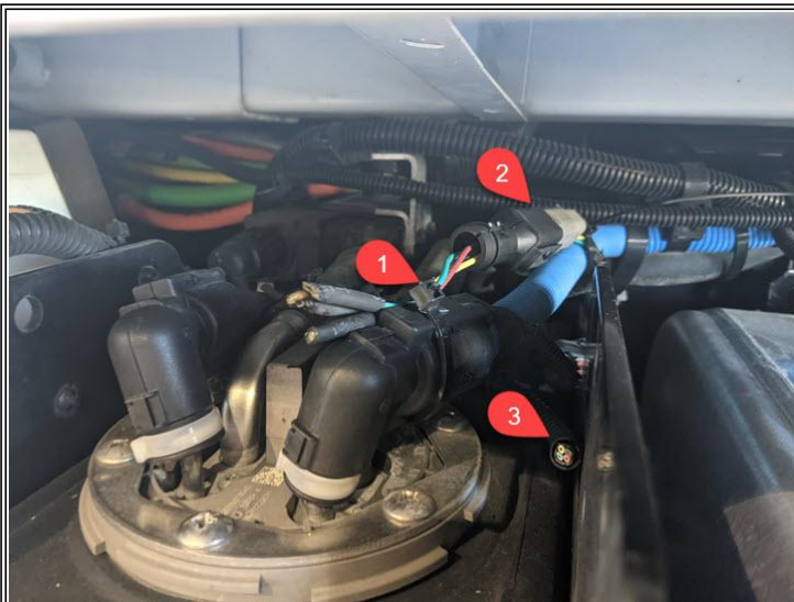
Figure 8: QLS Pigtail Installed
