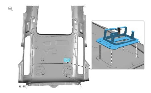
Using a suitable trim tool, carefully remove the <u>RF</u> receiver mounting bracket from the headliner.
