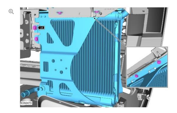
Install the new auxiliary radiator fixings.
