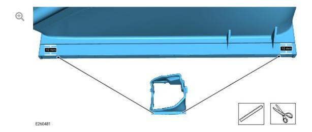
Modify the auxiliary radiator duct using the measurements illustrated as a guide. Step 8 shows a 'before' image and an 'after' to also be referenced.
