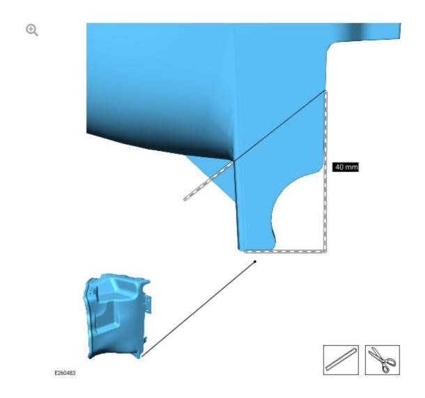
Modify the auxiliary radiator duct using the measurement illustrated as a guide. Step 6 shows a 'before' image and an 'after' to also be referenced.
