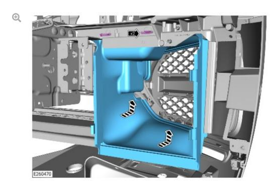
Install the modified auxiliary radiator duct.
