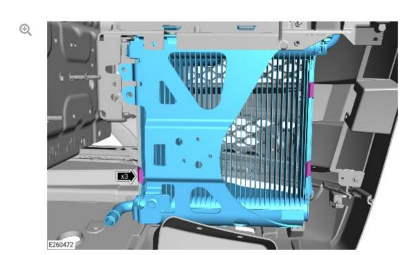
Install the new auxiliary radiator, making sure the 3 clips are correctly installed.
