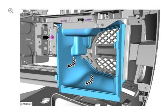
Remove and discard the auxiliary radiator duct.
