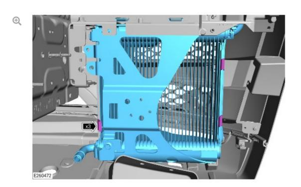
Install the new auxiliary radiator, making sure the 3 clips are correctly installed.
