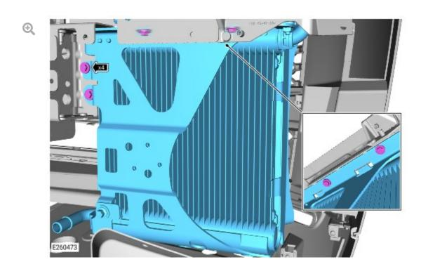
Install the new auxiliary radiator fixings.
