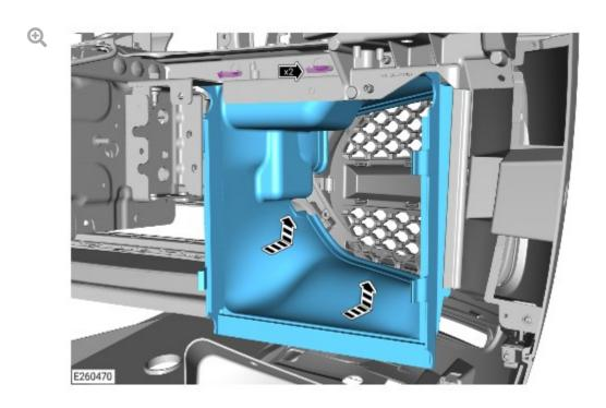
Install the new auxiliary radiator duct.
