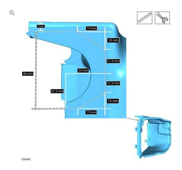
Modify the auxiliary radiator duct using the measurements illustrated as a guide. Step 4 shows a 'before' image and an 'after' to also be referenced.
