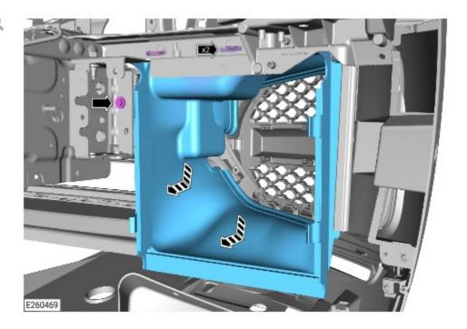
Remove the auxiliary radiator duct.
