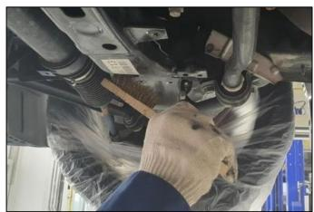
Use a wire brush to clean the brake banjo bolt surfaces at all four calipers and brake tube fasteners.
