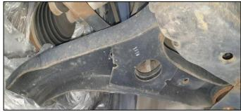
Rear Coupled Torsion Beam Axle (CTBA)
