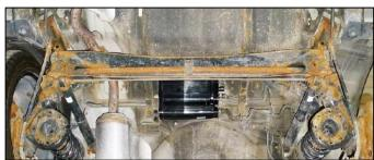
3. Use a wire brush to remove debris from the front sub-frame, left and right front lower control arms, and rear CTBA.
