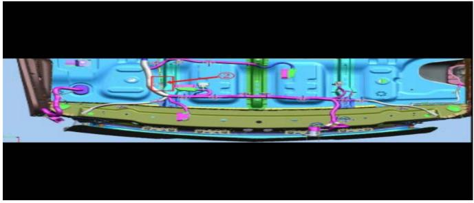
**Note:** The above view is from the underside of the rear body. The vehicle would need to be positioned on a hoist to inspect this connection location.
